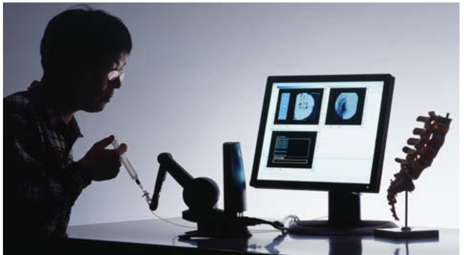
A device that simulates injection of fluid in the spinal cord
